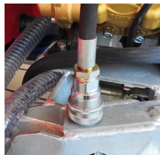
Hydraulische Bremsanlage Impianto frenante idraulico Hydraulic braking system
